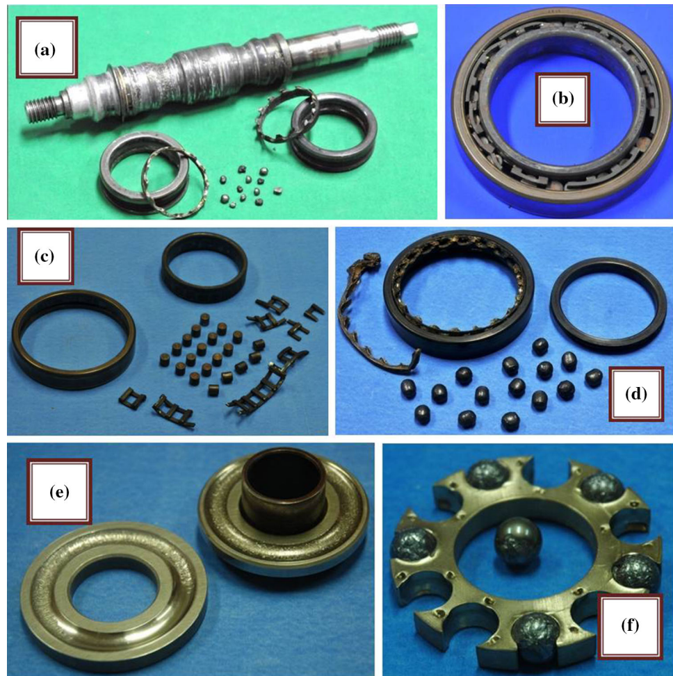
Fig. 1 Photographs of the failed components of various bearings in as-received condition: (a) bearing B-1, (b) bearing CMB-1, (c) bearing CMB-1, (d) bearing CMB-2, (e) EDP-1 and (f) EDP-1
