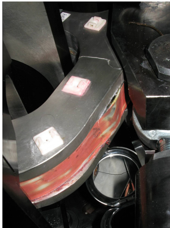
Fig. 5. The crack on the whole titanium section; the upper side and the lower side (in the mirror).
