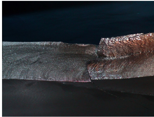
Fig. 3. View of the crack on the runner with the beach marks.
