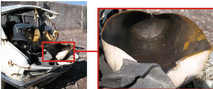
Fig. 2. Left: the wreckage of the car after the explosion. Right: the ruptured CNG tank. No burn mark was found on the wreckage.
