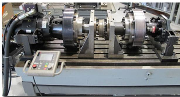
**Fig. 1** Torsional fatigue system
