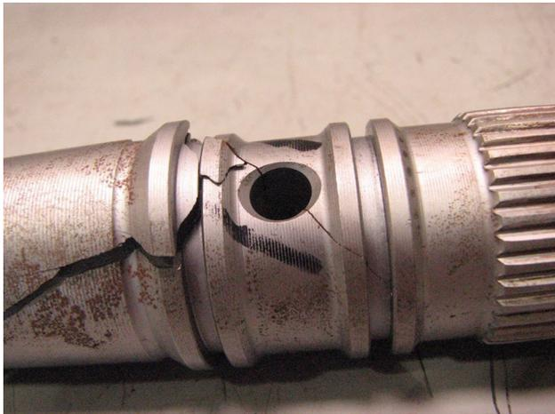
**Fig. 2** Macroscopic upper view of the fracture surface of the failed shaft which shows torsional fatigue fracture with fracture face 45° to the shaft
